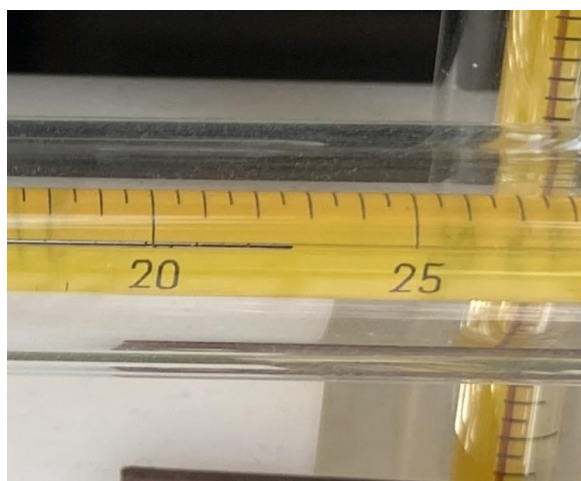
Mercury thermometer reading of the maximum temperature (22.6°C) recorded on the 30 th March, the warmest March day in the RMS record. Photo Credit: David Crowhurst.
