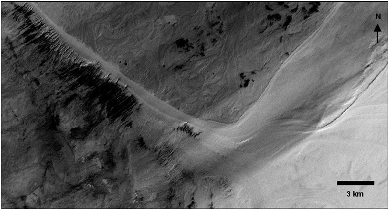
Figure 6 Landsat Band 4 image of the Angamma delta showing braided river channels on the delta top. The delta has a cusped morphology typical of wave-modified deltas and a well-defined beach ridge or beach ridge along the top of the delta front. The pristine preservation of the delta top and lack of incision through the beach ridge along the top of the delta front indicate that there was no low-stand or falling stage incision and that fluvial discharge ceased before the lake level fell. However, the base of the delta front is cut by gullies on its western side. This gully formation is attributed to groundwater sapping. We suggest that although surface water discharge on the delta top had ceased there was still some flow of groundwaters into the lake basin with subsurface flow emerging at the base of the delta deposits
